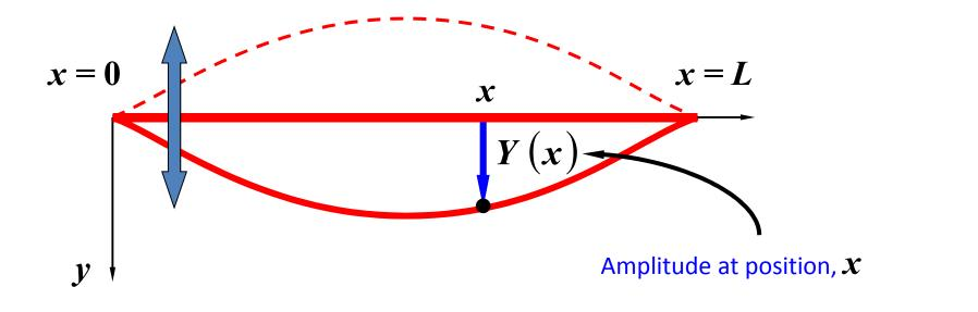
• Substitution of  $y(x,t) = Y(x) \cos \omega t$  into  $EI \frac{\partial^4 y}{\partial x^4} = -\rho A \frac{\partial^2 y}{\partial t^2}$
